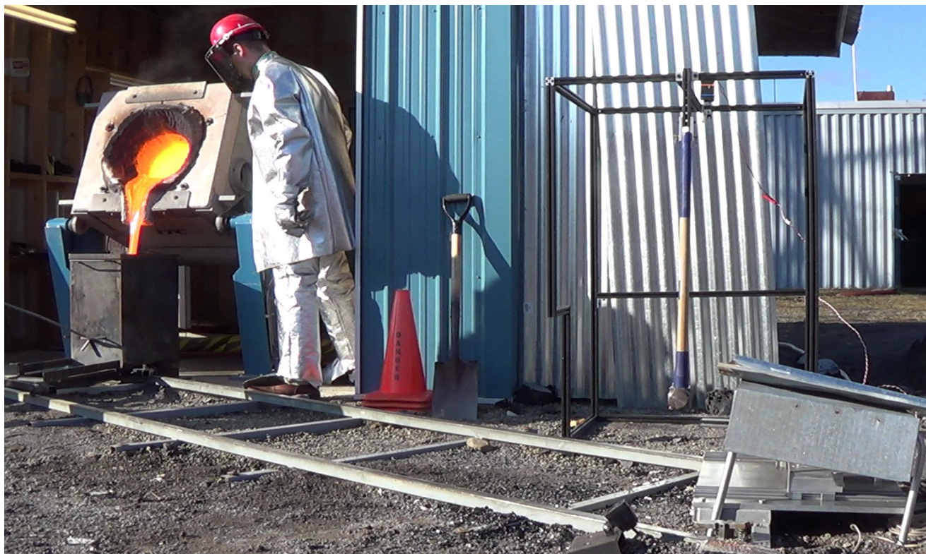
Experiment preparation. Melt is poured into the experiment container (left). The container is then moved on tracks to the water injection position (partially visible on the right).
