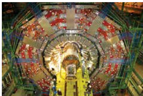
The CMS detector during the construction phase. Bright spots/mirrors serve as reference points for a precise laser alignment system. Photo: CERN
