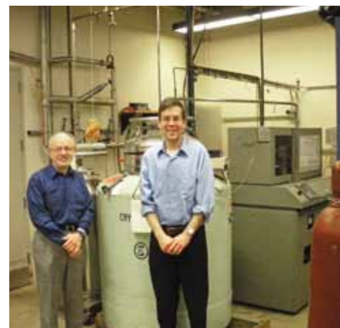
Former Cryogenics Facility director Dr. Frank Gasparini (left) with current director Dr. John Cerne in front of the helium liquefier. The olive-drab boxlike instrument on the right cools and compresses helium gas into liquid, which is then collected in the 500 liter dewar in the center of the photo. Photo: J. Wolf
